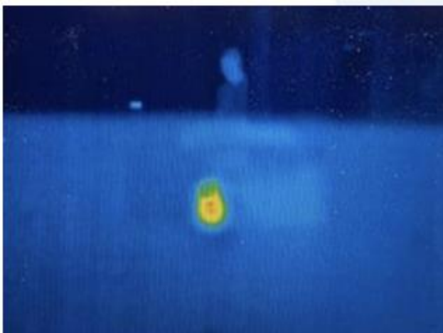
Figure 16. Thermal image of a cable showing a heat source at 124.2 °C.
